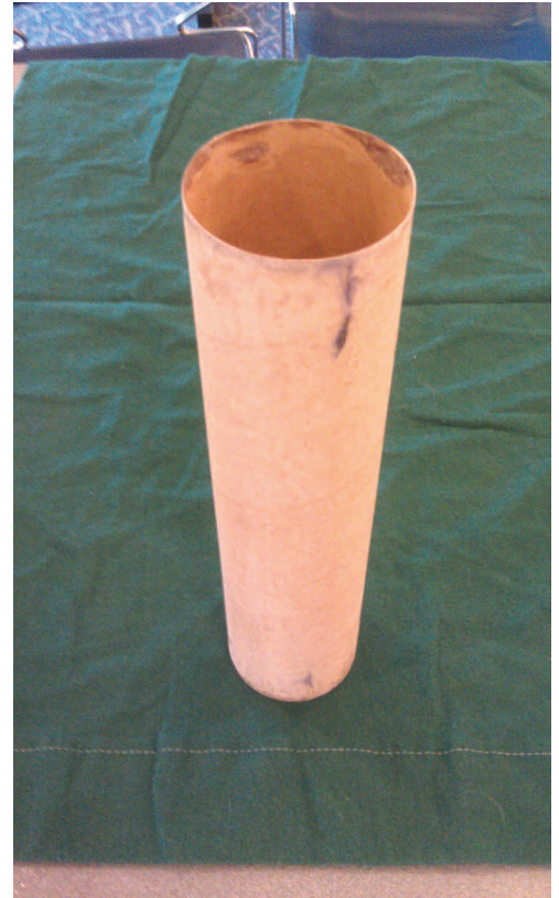
A glassed body tube. It's still very lightweight and smooth!
